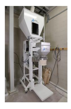
The Taylor Model APO is designed to fill open mouth bags with powder products that are aerated, bind, cake or bridge easily. The variable speed auger option utilizes Taylor's bulk and dribble technology and ensures a fast and accurate weight measurement while the inflatable spout creates a dust-tight seal on bags while filling. This unit comes with a hopper, the optional stainless steel contact surfaces, and food grade finish.
