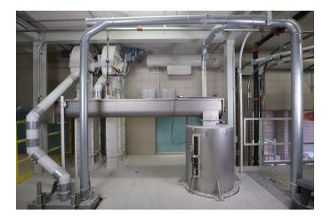
The Bühler Grain Tempering System is contructed from stainless stel and includes the Bühler MOZF-315C LC Semi-Automatic, Moisture Addition System.
