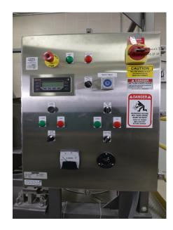
The A&J Mixing Co. Inc., PHLAUER™, Single Rotor Mixer is constructed from stainless steel. Most products can be mixed in less than one minute. The unit has a self-contained mixing system, with control panel and castor wheels for moving when not in use. The mixer is mounted on load cells for weighing amount of material added to the mixer. Additionally, the mixer has pneumatic knife gates above and below to fill and discharge the mixer.
