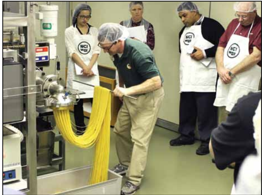
Rilie Morgan, NCI Processing Specialist, demonstrates how the pilot-scale pasta processor extrudes long-goods pasta that is caught on rods to hang in the dryer.
