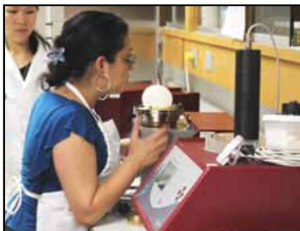
A participant learns to operate the Alveograph, which measures wheat gluten quality.
