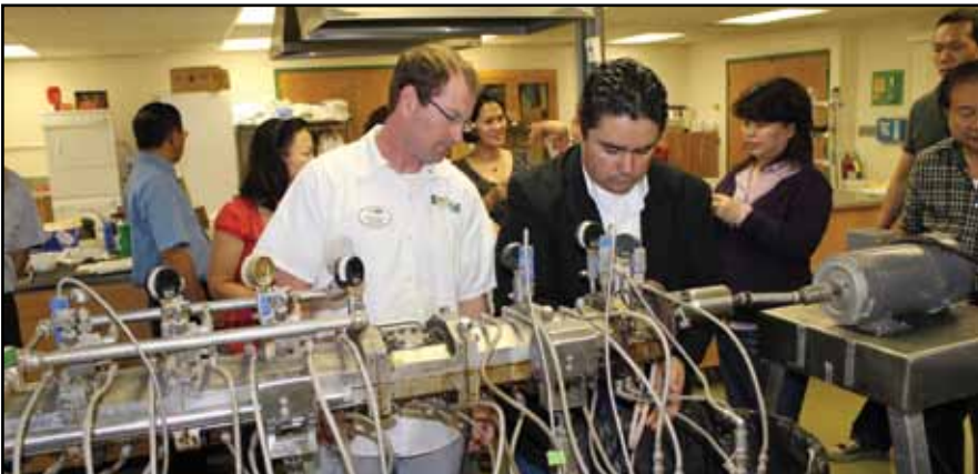
Rilie Morgan, NCI Processing Specialist, and Mehmet Tulbek, Ph.D., former NCI Technical Director, demonstrate the use of edible bean flour in extruded snacks using the NCI twin-screw extruder.
