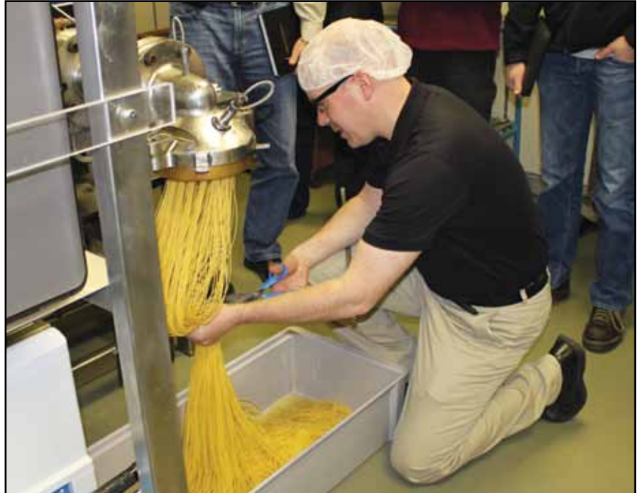
A participant catches spaghetti as it comes out of the pasta extruder.
