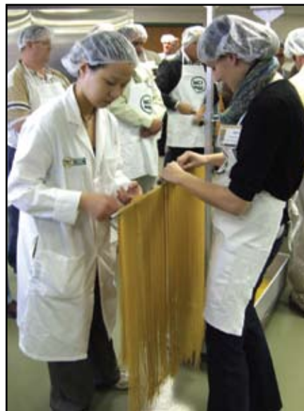
Naggie Jeradechachai, NCI Crop Quality Specialist, (left), assists a short course participant in arranging long goods before placing them into the dryer. The pasta was made on NCI’s pilot-scale pasta extruder during the class.
